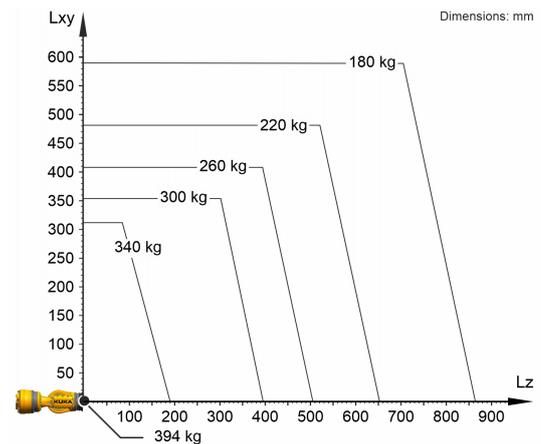
The KR 300 R2800-2 MT is designed for a rated payload of 300 kg in order to optimize the dynamic performance of the robot. With reduced load center distances and favorable supplementary loads, a maximum payload of up to 394 kg can be mounted. The specific KUKA Load case must be verified using KUKA. For further consultation, please contact KUKA Service.
