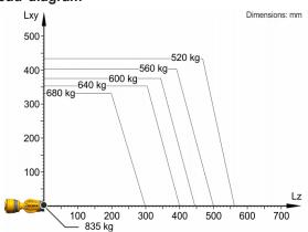
The KR 640 R2800-2 HI is designed for a rated payload of 640 kg in order to optimize the dynamic performance of the robot. With reduced load center distances and favorable supplementary loads, a maximum payload of up to 835 kg can be mounted. The specific KUKA Load case must be verified using KUKA. For further consultation, please contact KUKA Service.
