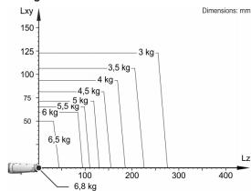
The KR 6 R700-2 EP is designed for a rated payload of 6 kg in order to optimize the dynamic performance of the robot. With reduced load center distances and favorable supplementary loads, a maximum payload of up to 6.8 kg can be mounted. The specific KUKA Load case must be verified using KUKA. For further consultation, please contact KUKA Service.
