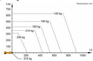
The KR 210 R2700-2 is designed for a rated payload of 210 kg in order to optimize the dynamic performance of the robot. With reduced load center distances and favorable supplementary loads, a maximum payload of up to 275 kg can be mounted. The specific KUKA Load case must be verified using KUKA. For further consultation, please contact KUKA Service.
