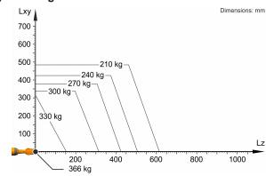
The KR 300 R2700-2 C-F is designed for a rated payload of 300 kg in order to optimize the dynamic performance of the robot. With reduced load center distances and favorable supplementary loads, a maximum payload of up to 366 kg can be mounted. The specific KUKA Load case must be verified using KUKA. For further consultation, please contact KUKA Service.
