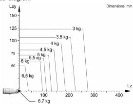
The KR 6 R900-2 EP is designed for a rated payload of 6 kg in order to optimize the dynamic performance of the robot. With reduced load center distances and favorable supplementary loads, a maximum payload of up to 6.7 kg can be mounted. The specific KUKA Load case must be verified using KUKA. For further consultation, please contact KUKA Service.
