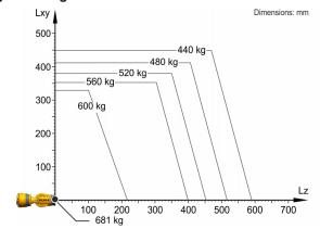
The KR 560 R3100-2 HI is designed for a rated payload of 560 kg in order to optimize the dynamic performance of the robot. With reduced load center distances and favorable supplementary loads, a maximum payload of up to 681 kg can be mounted. The specific KUKA Load case must be verified using KUKA. For further consultation, please contact KUKA Service.
