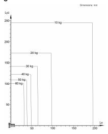
The KR 60 R1200 Z400 is designed for a rated payload of 20 kg in order to optimize the dynamic performance of the manipulator. With the reduced load center distances, higher loads up to the maximum payload may be used. The specific load case must be verified using KUKA.Load. For further consultation, please contact KUKA Support.
